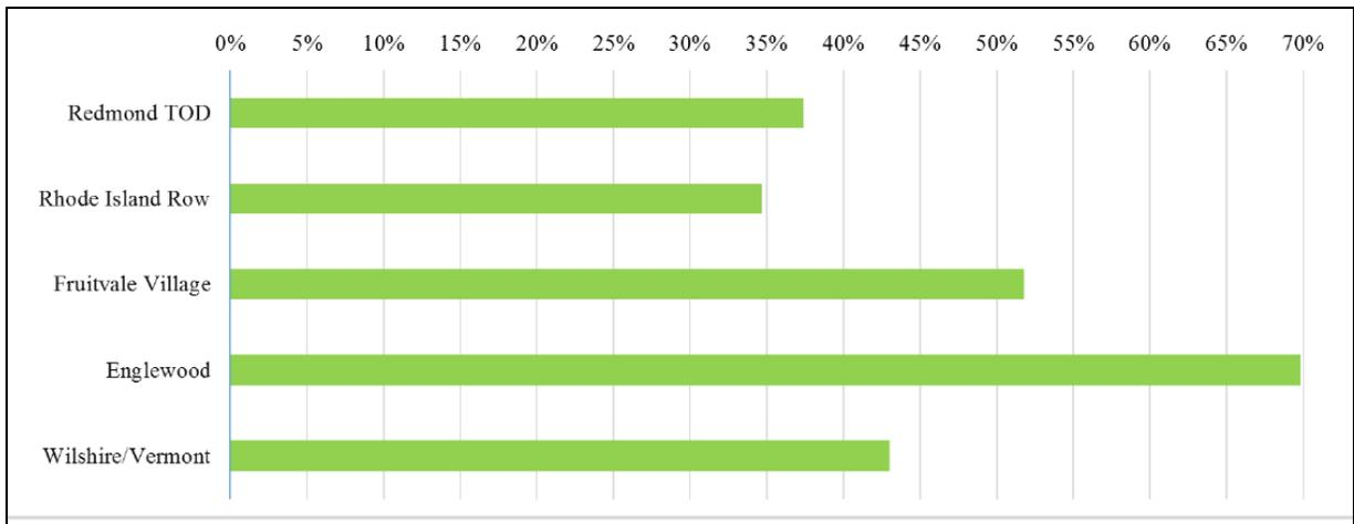
**Figure 11 Vehicle trip rates as percentage of ITE rates**
